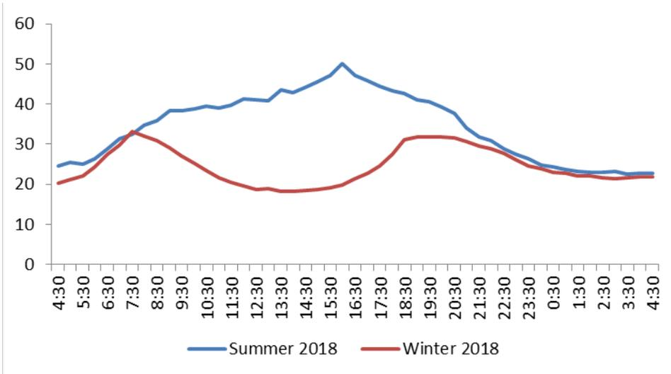
With increasing ‘behind the meter’ solar penetration, the profile of demand in Alice Springs for energy drawn from the grid is changing, with peak demand shifting to coincide with the start and end of the day (as solar generation ramps up or down). The level of demand drawn from the grid during the day is also declining (accentuating the curve seen in Figure 2) as demand is increasingly met from solar generation.
